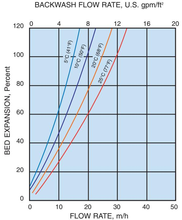
During upflow backwash, the resin bed should be expanded in volume by between 50 and 75%, in order to free it from any particulate matter from the influent solution, to clear the bed of bubbles and voids, and to reclassify the resin particles as much as possible, ensuring minimum resistance to flow. Backwash should be
